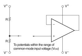
**Remark** A midpoint potential of V<sup>+</sup> and V<sup>-</sup> is applied to this example.
